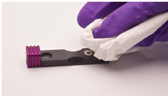
Cleaning BioDrop between DNA measurements
