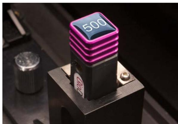
BioDrop 500 being used in an S60 Spectrophotometer
