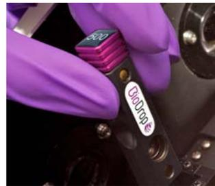
Light shines through the device and the optical path length of the measurement area is defined by a precisely machined spacer ring which is mounted on a thin membrane.
