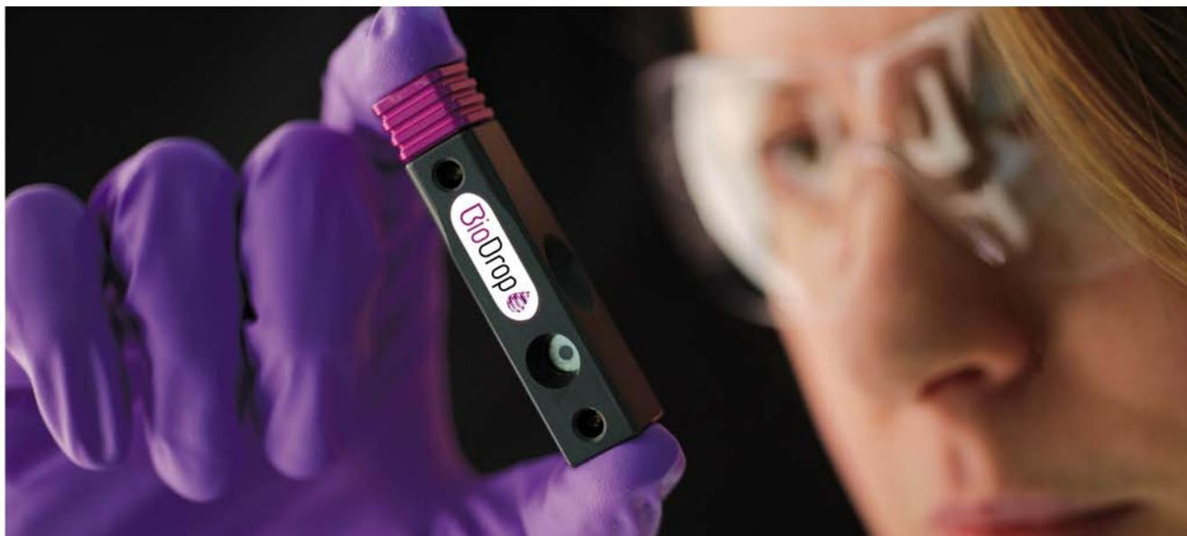
Spectrophotometry remains one of the simplest ways to perform colorimetric assays in a laboratory environment. For the molecular biologist, absorbance measurements at 260nm provide a simple way to measure DNA concentration. The ratio of absorptions at 260nm vs. 280nm is commonly used to assess DNA contamination of protein solutions since DNA absorbs light at 260nm, and proteins (in particular, the aromatic amino acids) absorb light at 280nm.
